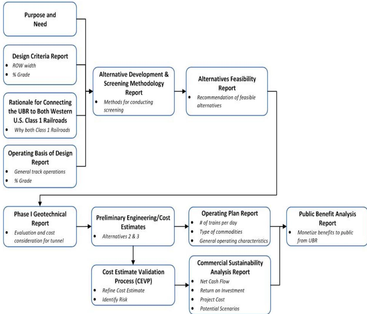
Phase 2 included conducting the environmental field surveys for the feasible alternatives and developing the baseline environmental discipline reports. Figure 3 below shows the process for developing this information.
